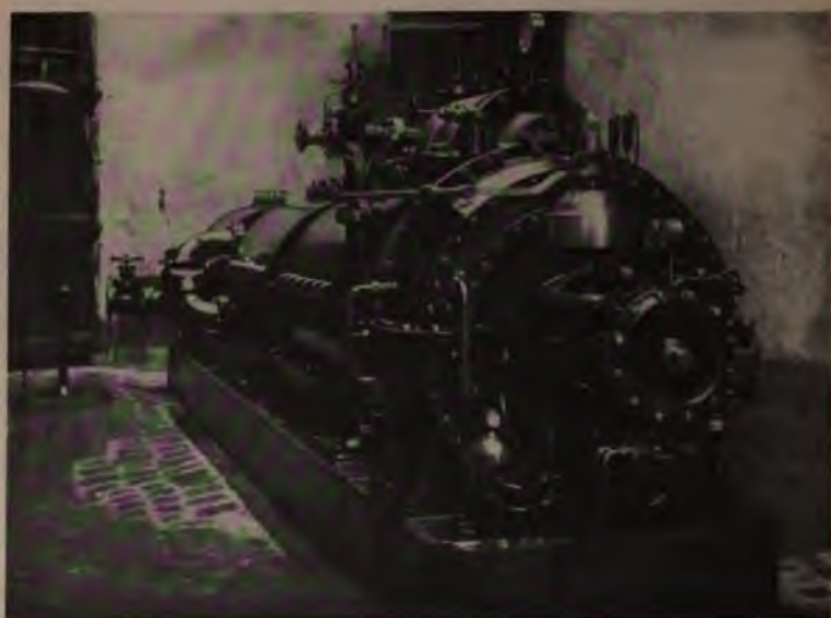
FIG. 90.—The 300 horse-power gas turbine of Armengaud and Lemale connected to the Rateau polycellular turbine compressor.
